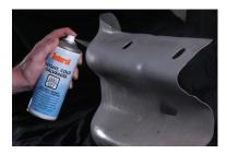
A single component, zinc-aluminium coating combining corrosion protection properties with the lustre look of recently galvanized parts. Bright Cold Galvanising Spray is a combination of zinc and aluminium powders, resins and additives, formulated to form a flexible protective film with a bright, glossy appearance.
